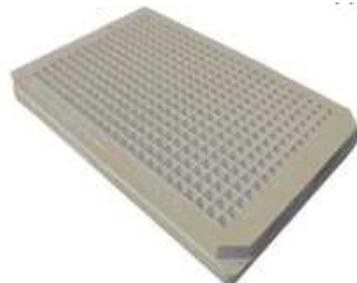
384-well plate: used by AccuFill™ System to transfer samples to OpenArray® plate
